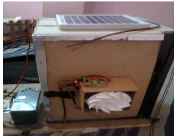
Fig 4: Working Model of a Compressor Less Solar AC
